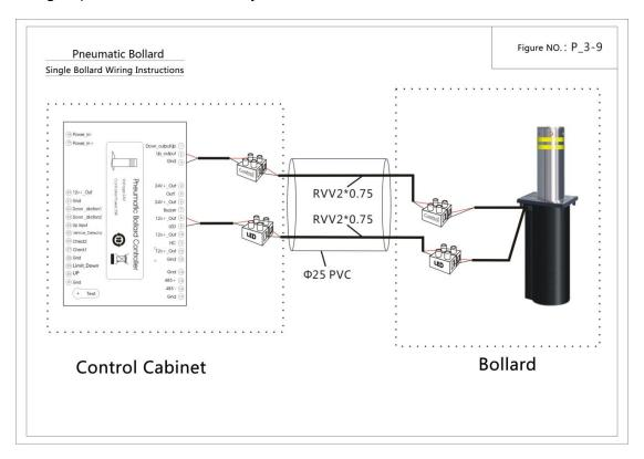
Instructions:  $\Phi$ 25 PVC pipe pre-buried as shown in the above diagram contains 2 lines and 1 air pipe  $\Phi$ 10. Air pipes of each bollard should be connected to the shunt inside the control cabinet.
