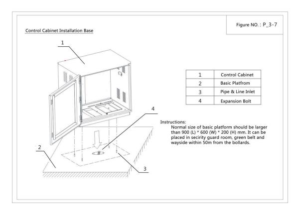
Lay a basic platform where the control cabinet is placed. Make the control cabinet 200-300mm higher than the ground to prevent unwanted influence caused by rainwater. The center part of the platform must be hollow for wiring and other work. Finally fasten it on the platform with 4 expansion bolts.
